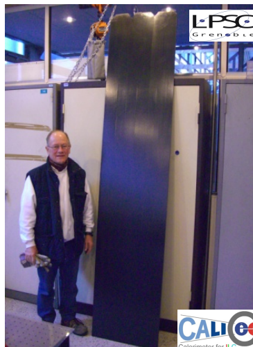
Moulding of one layer / 3 alveoli L = 2.490 m wall thick. = 0.5mm
