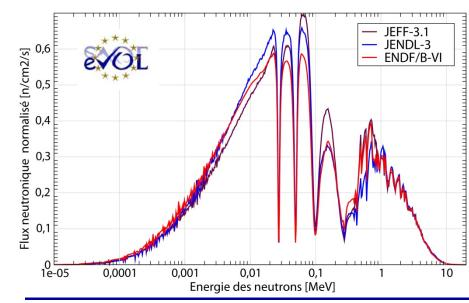
LPSC-IN2P3 calculations performed with MCNP (coupled to in-house material evolution code REM)
