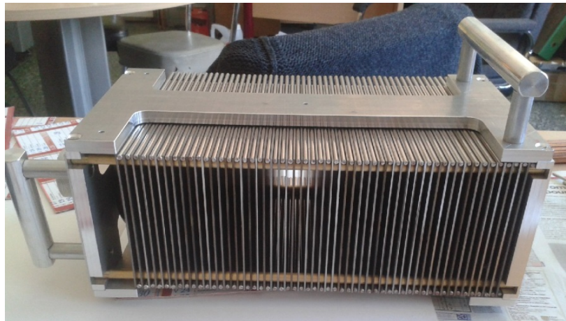
Tungsten alloy collimator (12x10x0.2 cm slabs)
