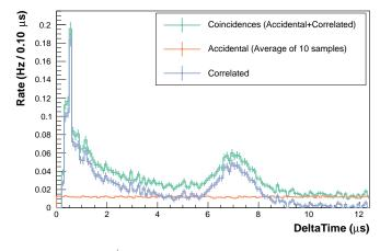
1st afterpulse at  $\sim 0.5\,\mu s$  :  $H^+$  2nd afterpulse between  $[6-8]\,\mu s$  :  $N_2^+$ ,  $Ar^+$ ,  $O_2^+$  or/and  $CO_2^+$  Exponential contribution ?
