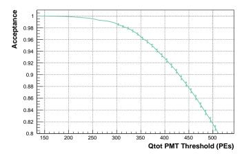
For threshold of [200-300] PEs  $\Rightarrow$  -0.1% / 10 PEs For threshold > 100 PEs  $\Rightarrow$  -1% / 10 PEs
