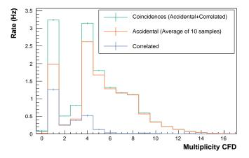
Expect afterpulse events to have a PMT multiplicity = 1 Cut on multiplicity > 1 should remove after pulse
