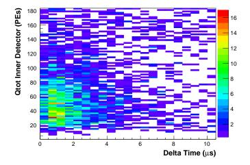
Cut on delta time  $\Delta T$  or cut on charge Qtot to reject correlated ?
