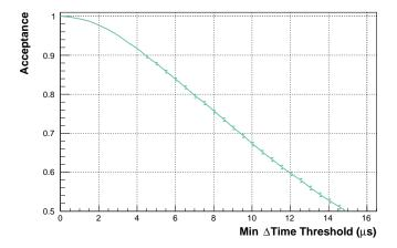
Cut on lower delta time threshold has a big impact on the neutrino acceptance
