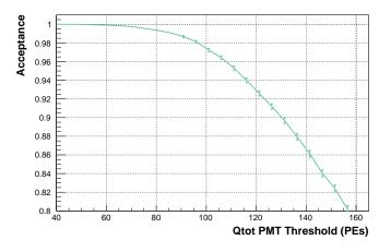
For threshold of [60-90] PEs  $\Rightarrow$  -0.5% / 10 PEs For threshold > 100 PEs  $\Rightarrow$  -2% / 10 PEs
