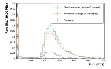
Peak at 500 PEs caused by muon going through veto muon  $\Rightarrow \sim 80\%$  of prompt events Some events don't produce any signal in veto  $\Rightarrow \sim 20\%$  of prompt events
