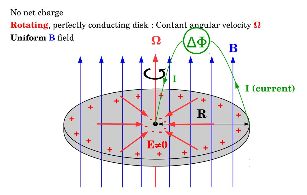
Induced electric field **E**=-**V**×**B**/**c**=-( $\Omega$ ×**R**)×**B**/**c**. The disk is **polarized**.
