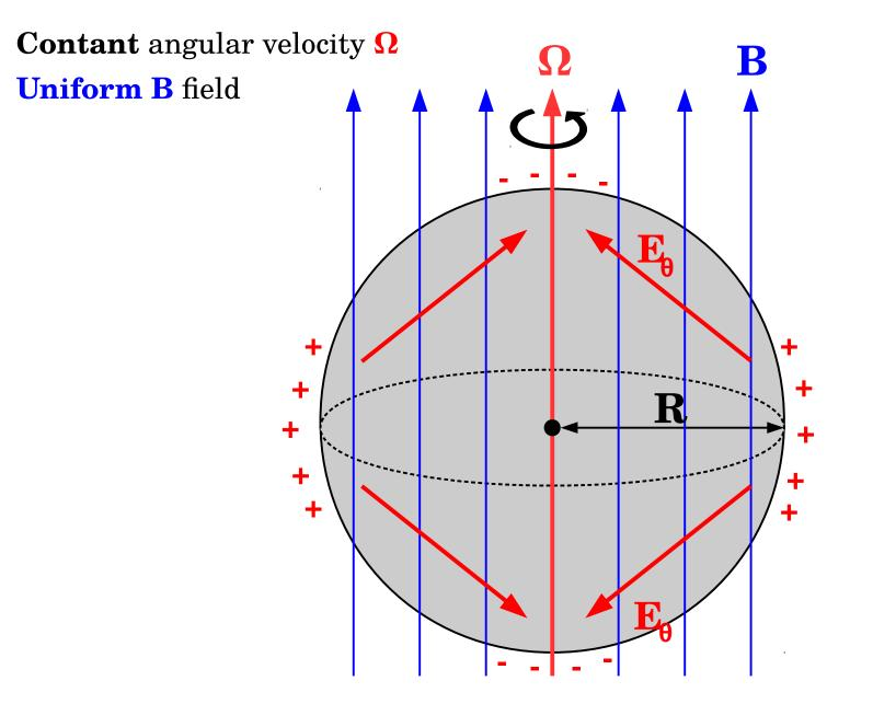
Induced electric field  $E=-V \times B/c=-(\Omega \times R) \times B/c$ . The sphere is **polarized**. => **Potential difference between the <u>poles</u> and the <u>equator</u>**
