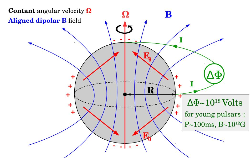
Induced electric field **E=-V×B/c=-(Ω×R)×B/c**. The sphere is **polarized**. **=> Potential difference between the <u>poles</u> and the <u>equator</u>**
