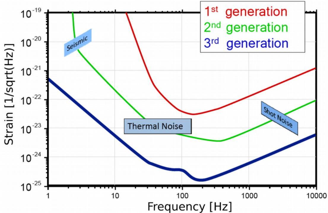
From Pushing towards the ET sensitivity using ‘conventional’ Technology - Stefan Hild et al. - arXiv:0810.0604v2
