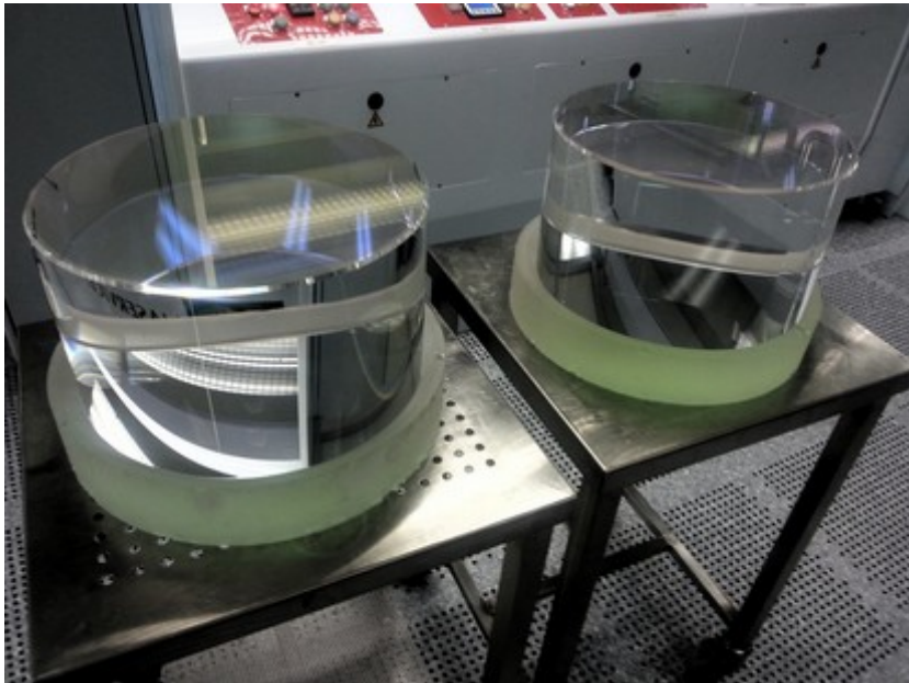
40 kg mirrors of Advanced Virgo 35 cm diameter, 40 cm width
