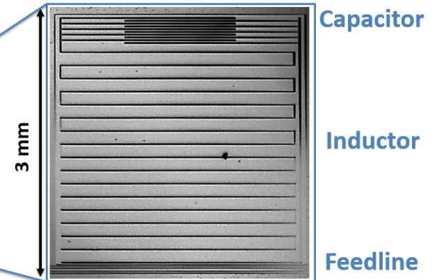
One of the 632 pixels within the KISS camera
