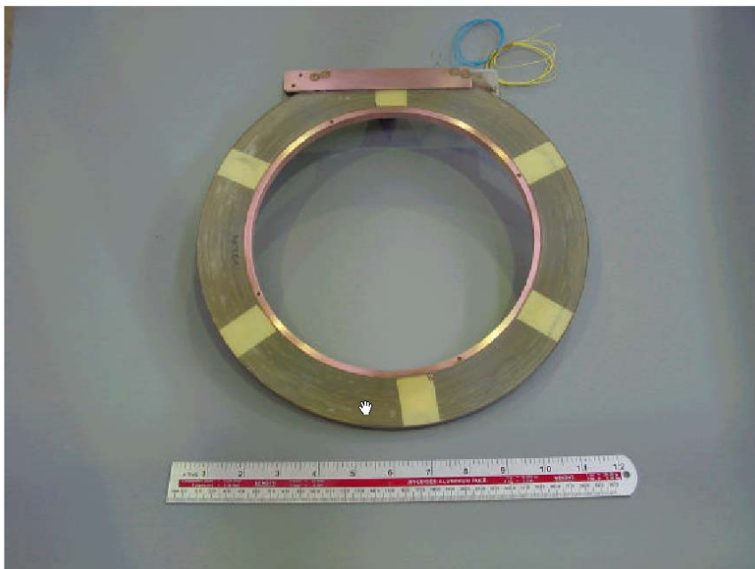
Figure 4: Finished prototype coil
