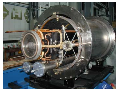
Nuclotron dipole magnet: B=2T , dB/dt=4T/s
