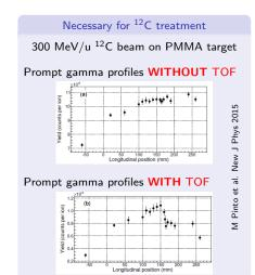
An external detector is necessary for multi-energy treatment (RF phase varies!).
