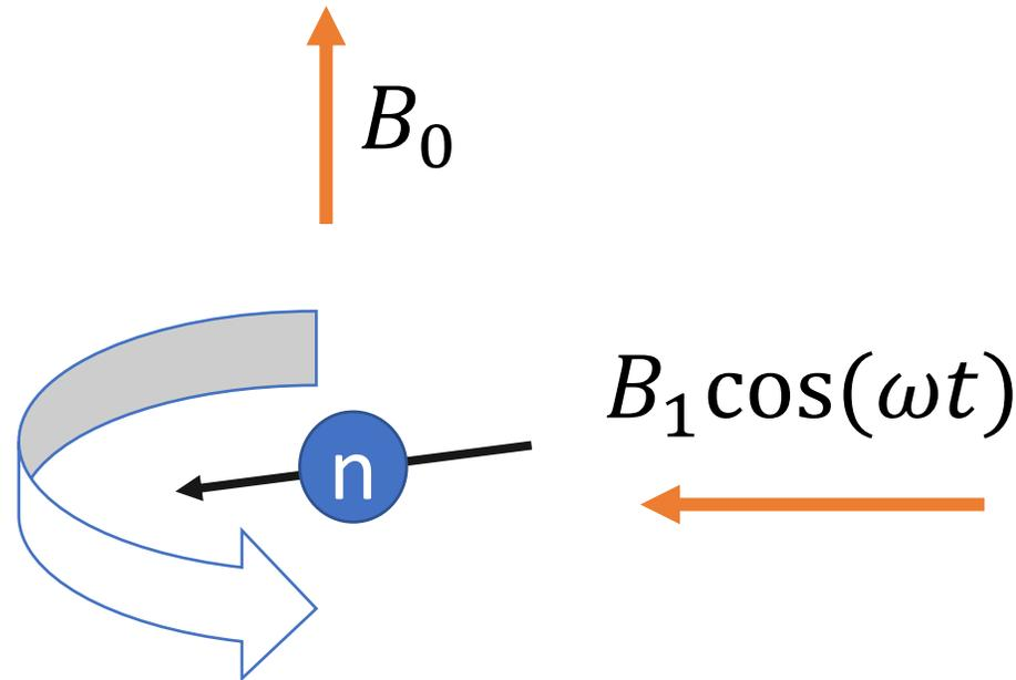
$$\gamma' \approx J_0 \left( \frac{\gamma B_1}{\omega} \right) \gamma$$
