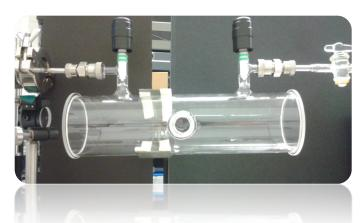
Crossed pump & probe beam configuration allows optical pumping, T<sub>1</sub> & T<sub>2</sub> tests, Rabi flopping, AFP
