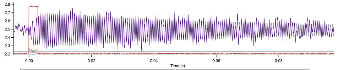
Obtained  $^{199}$ Hg FID signal at  $^{200}\mu$ T with n=100 averages Study the dependence on  $\pi/2$  pulse parameters and on inhomogeneous  $B_0$  field:
