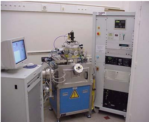
Plassys: metal deposition device at NanoFab NanoFab is a platform of Institut Néel
