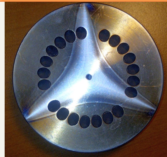
Erosion of the plasma electrode shows plasma symmetry
