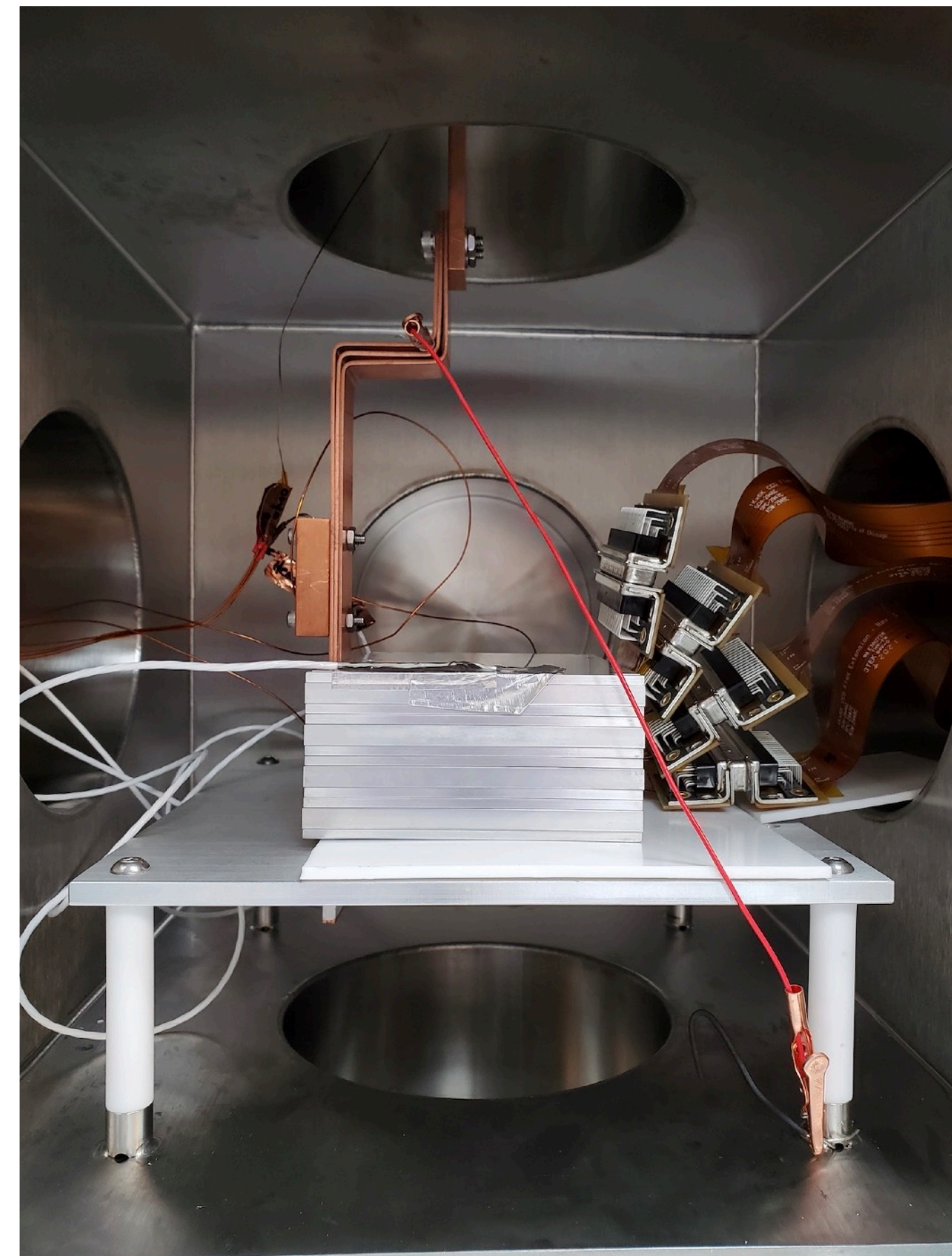
Vacuum chamber with four CCDs
