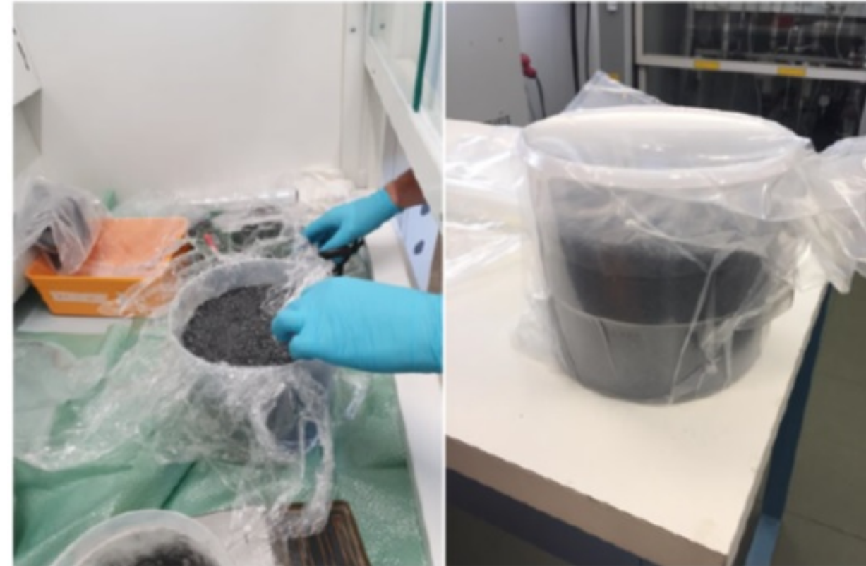
Sample of enriched ^{82}\text{Se} (enrichment \sim 95\% ) with a mass of 6019.9 g of ^{82}\text{Se} was prepared in Marinelli of Obelix detector in LNGS in July 2020.
