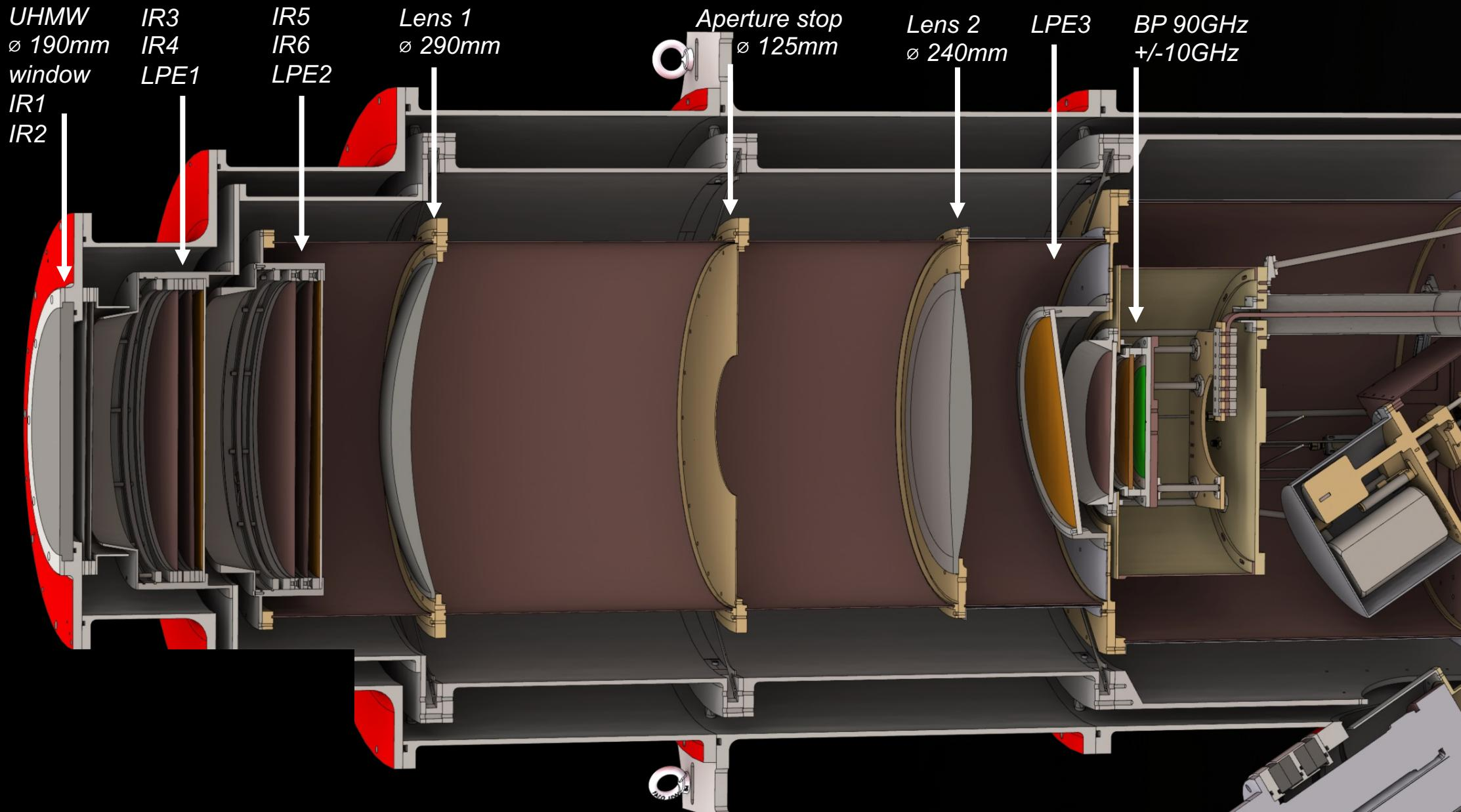
Combination of: Metal mesh filters, thin IR filters, sub-mm low pass filters (LPE), a final 74-103GHz Band pass filter
