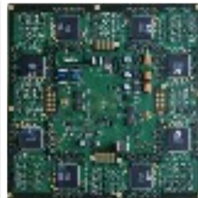
Micromegas 10x10 cm 2 , designed by IRFU- Saclay (France)
