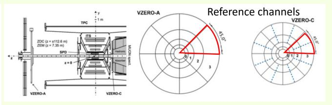
Equalizate gain to uniform the each channel value on the same ring.
