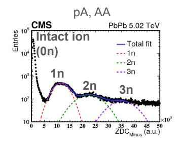
Tagging neutron emissions from giant dipole resonances (Zero degree calorimeters in CMS, ATLAS, ALICE, STAR)
