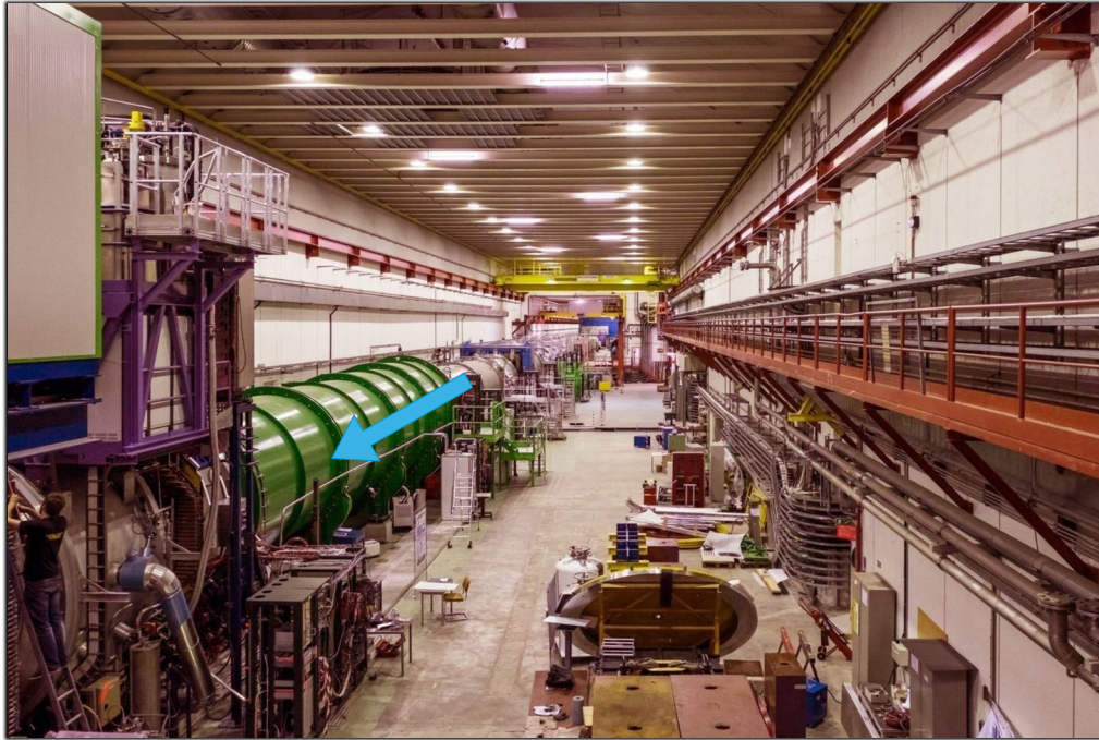
NA62 experimental hall from downstream. Green detector is the RICH. Arrow indicates the beam direction.
