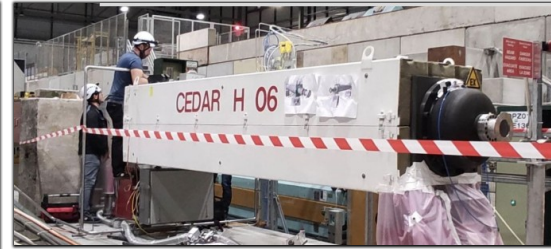
The upstream tagging Cherenkov detector (CEDAR)
