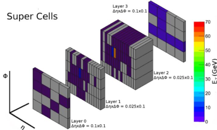
≈ 10-fold increase in granularity (5k trigger towers → 34k Super Cells)
