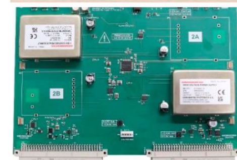
HV Supply Board
