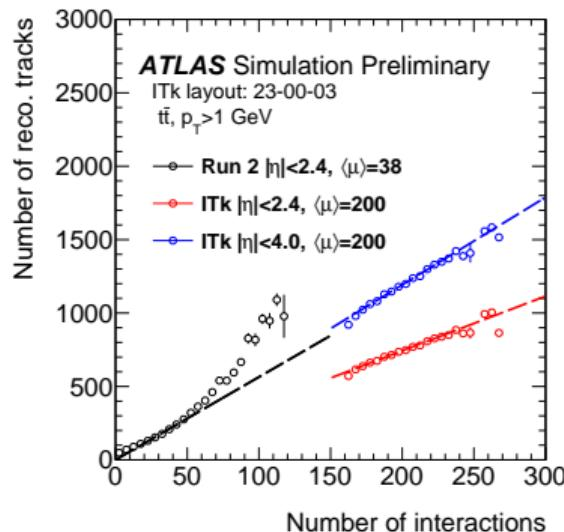
→ Robustness of the tracking efficiency over a large pileup range, thanks to the deployment of an optimised seeding strategy + hit requirements
