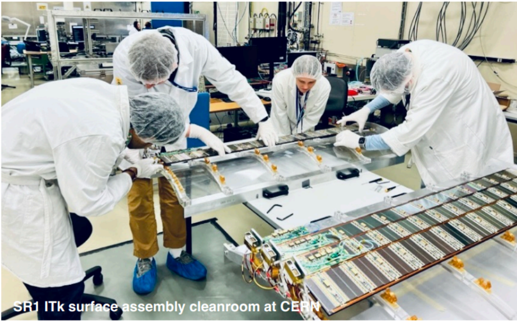
Full-scale barrel IS integration mockup
