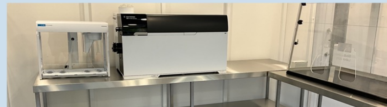
ICP-MS (Surface): Newly installed system for trace element analysis and isotopic ratio measurements.
