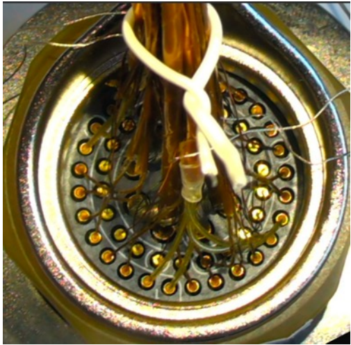
Prototype #2 before potting
