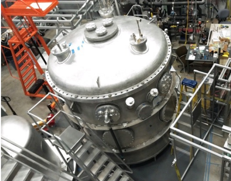
Magnet system closed for cold test at ORNL
