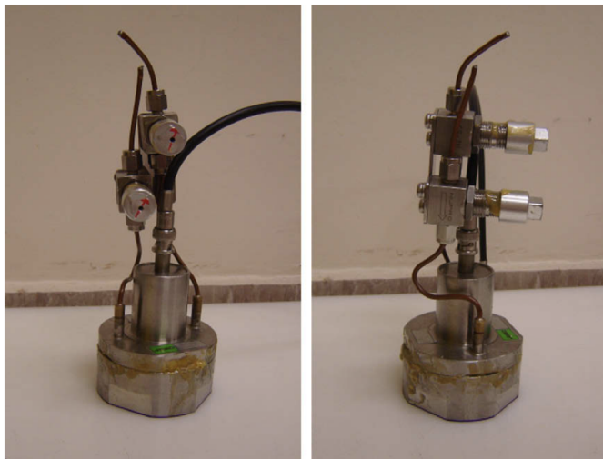
Fig. 1. Front view (a) and side view (b) of the Cf source-detector.
