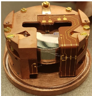
Fully Inter-Digitized (FID) electrodes :
