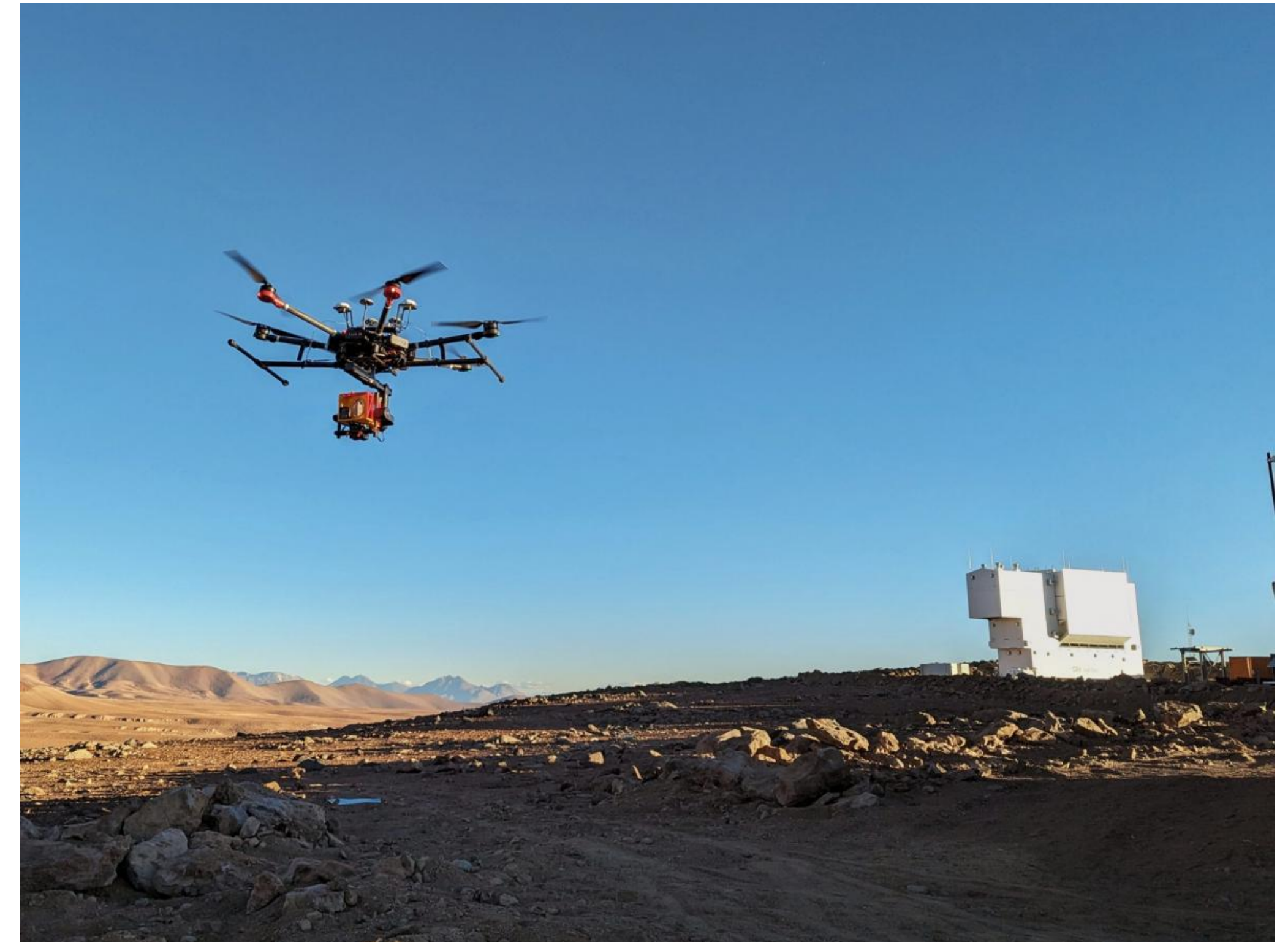
POLOCALC drone used for calibration of SO-SATs & CLASS in the Atacama desert
