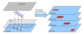
ullet Multiplexed strip readout o each time slice picture is rectangular
