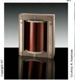
60 kVA Demonstrator 1kV/0.6 kV Primary copper Secondary YBCO tapes Successful test in 2010 Recovery under nominal load 2 MVA Demonstrator
