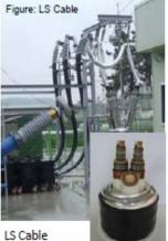
22.9 kV, 50 MVA, 100 m BSCCO 2223 Energized 2007 500 m field test with YBCO in 2011
