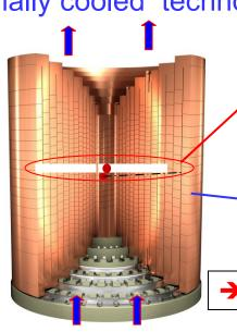
Heat conduction length = helix thickness
