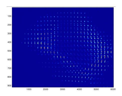
Single beam lets on a viewing target coming from an analyzed ion beam (one charge state only) defined by a pepper plate.
