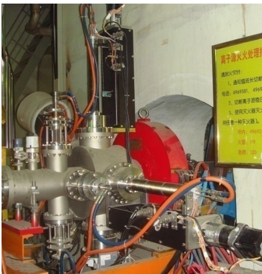
IMP Allison-type emittance scanner. Located after the analyzing magnet
