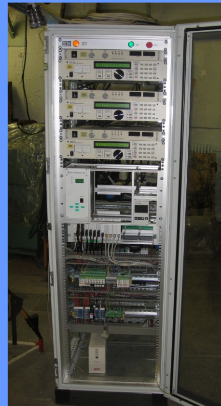
Power supply and control system of SC magnet
