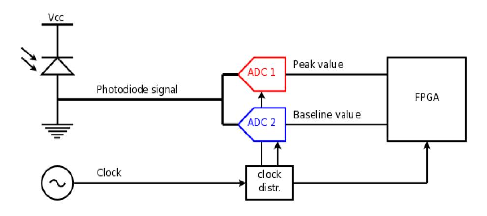
Signal distribution with 2 ADCs - "T" distribution is weak point
