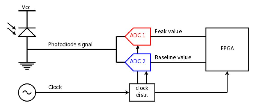
Signal from photo diode is sampled using two ADCs, with clock signal shifted in phase
