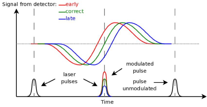
The amplitude of the correct in time bunch is same as the amplitude of the unmodulated pulses, due to zero-crossing
