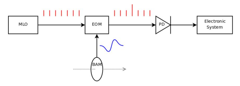
Amplitude of laser pulses generated by the reference synchronization system (MLO) is modulated by the arrival time of the traveling bunch
