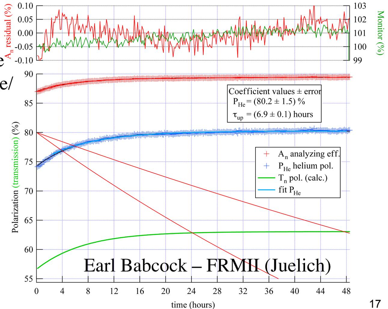
$^3\text{He}$  spin filter  $n+p \rightarrow d + \gamma$  (@LANSCE)
