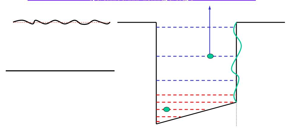
The wave functions for the upper levels reach the rough wall. After collisions, the particles can go above the threshold and disappear. The wave functions for the lowest level particles do not reach the rough wall. Only these particles will survive the scattering!
