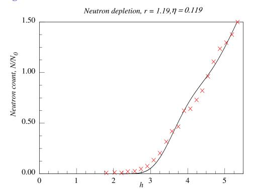
"Old" GRANIT cell. The roughness is assumed to be 1D with Gaussian correlations; r = 1.19,  $\eta = 0.119$ . The value of  $\Phi = 23.5$
