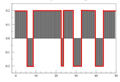
Element of an "Ising" mirror: red lines- mirror surface, grey bars – Ising "spins" ( $\sim 6 \mu$  wide)
