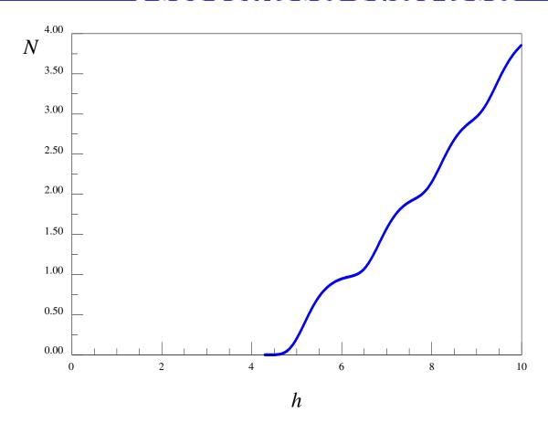
Predictions for the "new" GRANIT cell. 2D roughness with the exponential correlation function with r = 0.65,  $\eta = 1.02$ . The correlation function was extracted from the experimental data on the surface profile.
