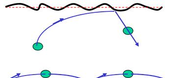
The particles with higher vertical velocity reach the upper, rough mirror and can acquire an even larger vertical velocity after scattering
